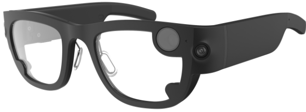
Figure 8. The Project Aria device used for egocentric recordings.
